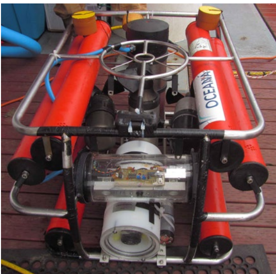
The team's Mariscope-FOII ROV was deployed to capture high-definition underwater footage
