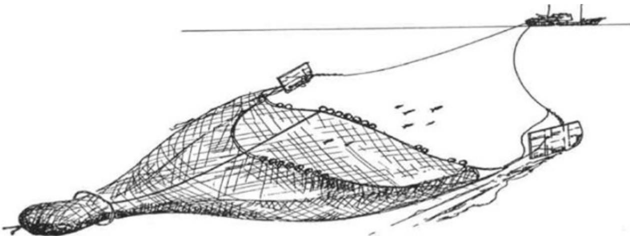
**Figure 1.5.** Bottom Trawl Fishery System (Courtesy NOAA).
